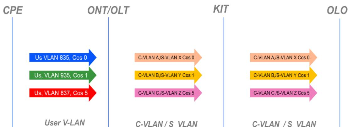
**Figura 11 – Modello VLAN Mono CoS Double Tag QinQ**
