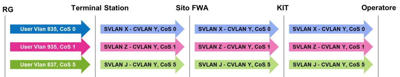
**Figura 18 – Modello VLAN Mono CoS Tagged OpenStream FWA**
