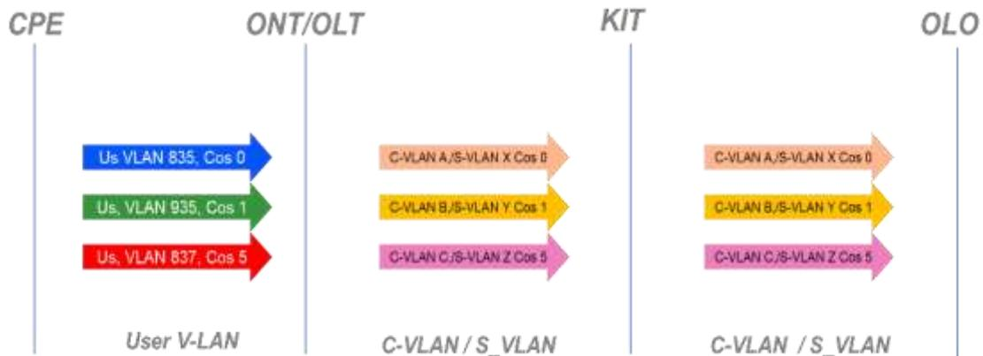
**Figura 9 - Modello VLAN Mono-CoS double-tag QinQ**
